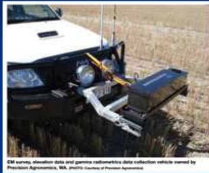
EM survey, elevation data and gamma radiometric data collection vehicle owned by Precision Agriculture, WA, Seattle (courtesy of Precision Agriculture)
