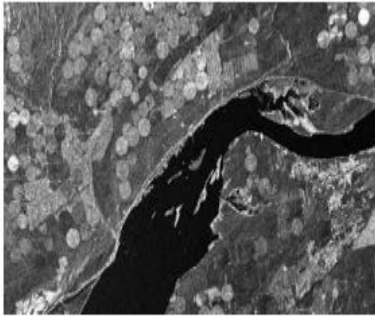
Figure 8. RADARSAT-1 image illustrating variations in backscatter due to pivot irrigation activities; higher soil moisture appear brighter.
